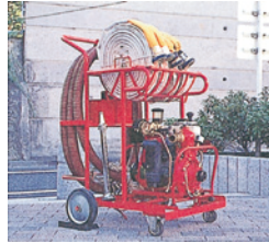
Small Fire Extinguisher Pumps
